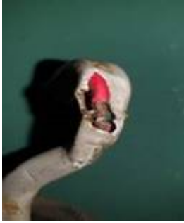
Damage to cable inside the column including evidence of previous repairs
