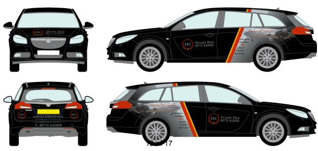
Materials & method proposal: Silver metallic high sparkle as a base, printed with the black shade effect & ghosted image of the 747 (overlaminated in clear high gloss All additional text / graphics will be over applied so as to assure accurate levels etc.
