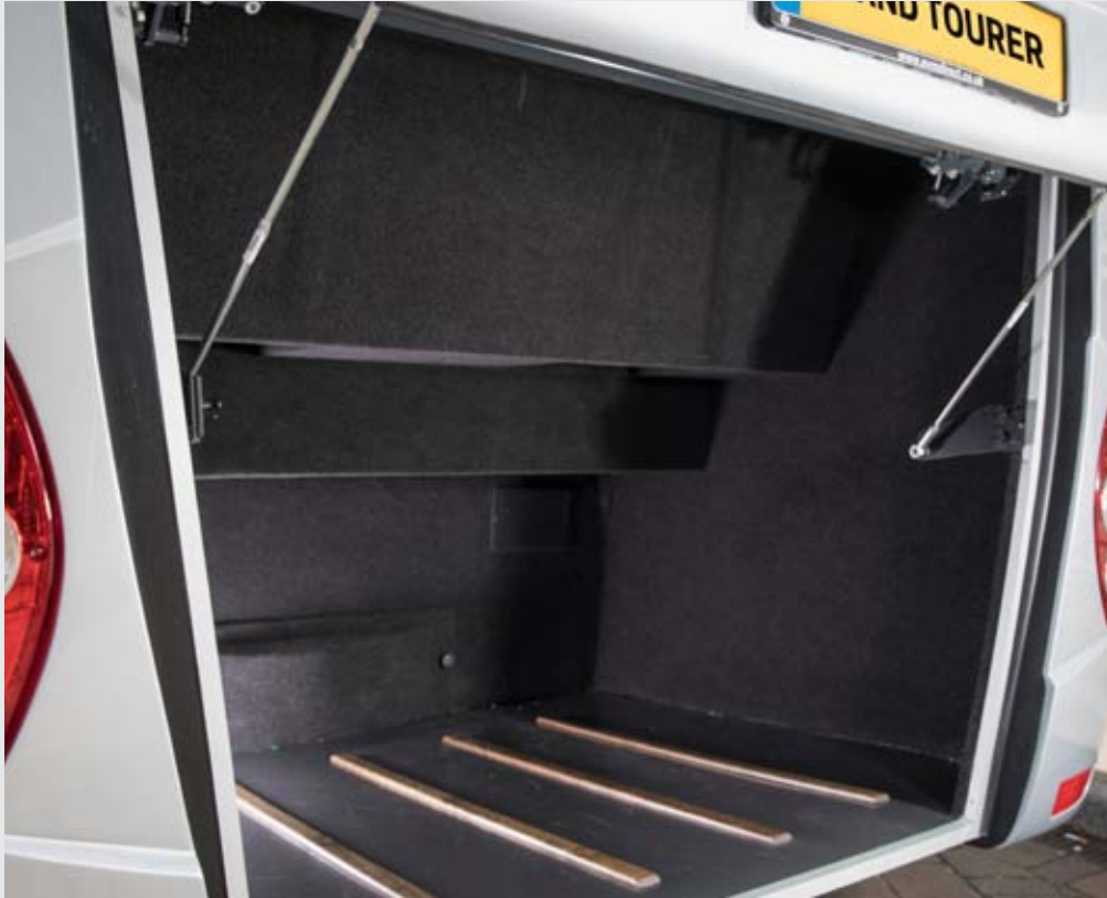
SPACIOUS, LUGGAGE STORAGE The coach back vertically elevating electrically powered door has an internal open and close switch which can only be accessed by the driver but does come with a manual override facility. The rear boot space will cater for a huge amount of luggage
