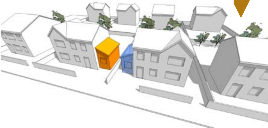
Design Guidance 2: Single Storey Side Extension to Two Storey Dwelling - Good Design Practice
