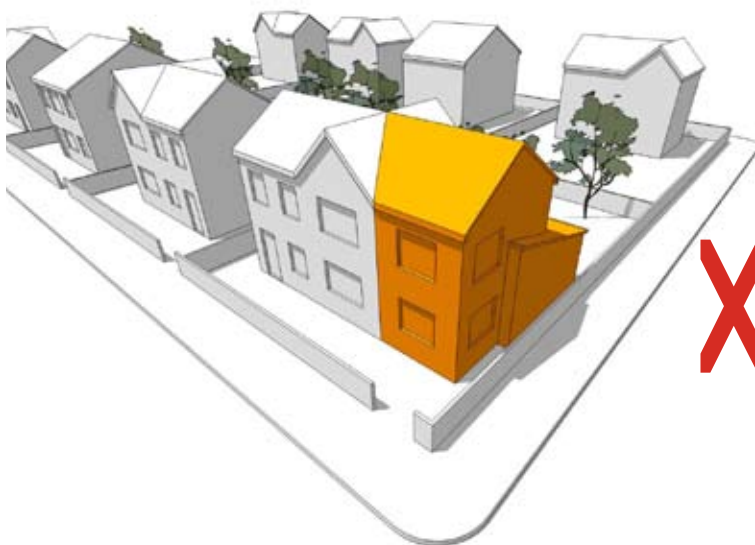
Design Guidance 7: Corner Extension Overly Dominant Poor Design Practice
